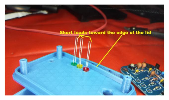
Tip the lid upside down and insert the LEDs in the holes as shown. Do not mix up the colors, red going near the center of the lid. Put the leads so that the short lead (and the flat side of the diode) is toward the side of the lid as shown.
