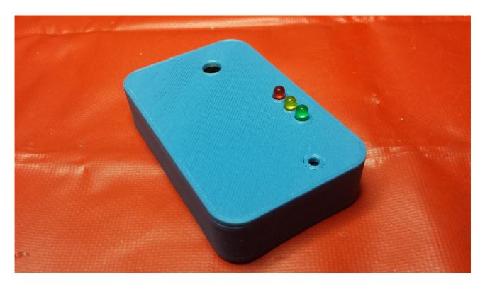
I have not added holes for the power leads, leaving them to be drilled by the user. We each may have our own requirements for connecting to the VT2. A little hot glue as a strain relief for the wires coming into the case may be a good idea.
