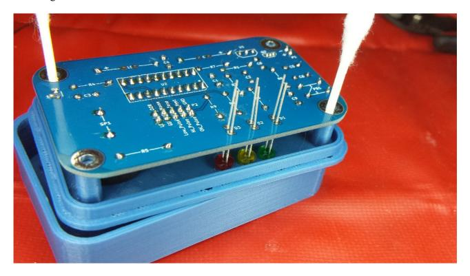
Next solder in the LEDs. Solder all 6 leads.
