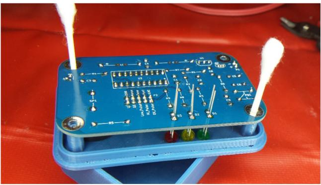
Then simply remove the centering tools (swabs in this case). There are no screws holding the board into the case. It is held by posts printed into the lid and base. He lid simply snaps on.
