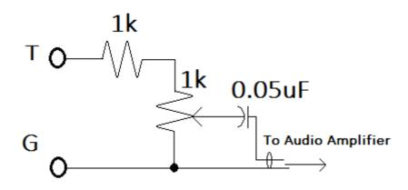
The above circuitry somewhat isolates the audio output from the microcontroller. It also provides a bit of adjustable attenuation for the audio. Be aware that AC hum may be present here in the form of ground loop hum. An isolation transformer can help. In addition amplification locally to VT can cut down on ground loop induced hum.
