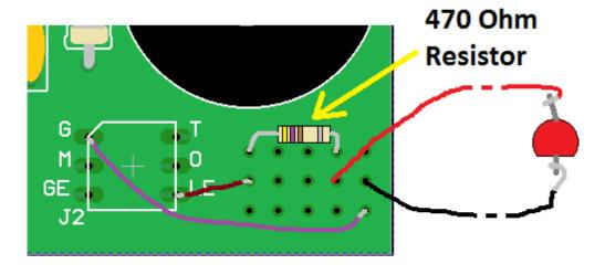
We see that a simple series resistor of 470 ohms is enough to allow the red LED to shine. A 270 Ohm resistor would be used to drive a green LED. But remember that whenever Volt Tattler is driving the LED, that current must be added to the total draw for the system.
