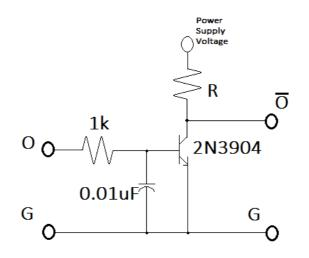
Any of the signals can be inverted simply with the circuit above. In this case the output logic level will be the inverse of O. This may be useful if a true logic signal is needed to indicate that the voltage is OK. Resistance and power values for R should be determined for driving downstream logic requirements. If we want to drive an LED, however, R can be determined as shown here.
