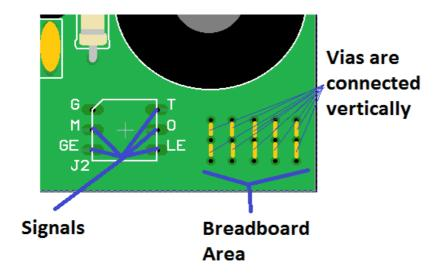
The Volt Tattler V1.01 has the signals next to a small breadboard area. It is hoped that this small area will assist in getting signals from the board for use by equipment downstream. The breadboard area is a set of vias vertically connected. Parts may be inserted here for experimentation and implementation purposes.
