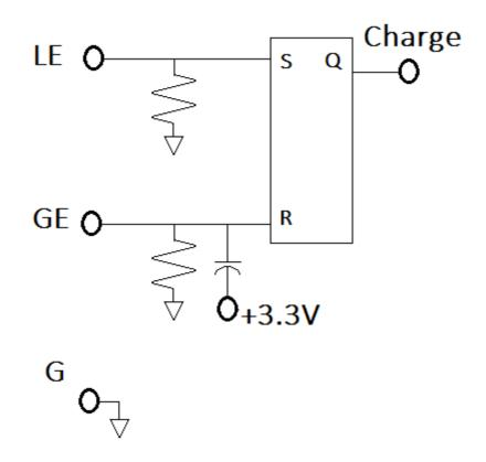
Essentially VT drives a Set/Reset flipflop. The HC logic family interfaces nicely here. The capacitor would force a reset at power up so that the unit will not start charging just because the R/S flip-flop saw power. This is just a suggestion. Considerably more work would be needed to provide a viable voltage controlled battery charging system.
