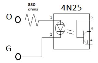
It is possible to optically isolate the output making it more immune to downstream common mode issues. Here the O output has been selected to drive a 4N25 optoisolator. With the 330 ohm resistor the LED should drive at about 5 mA. With the 4N25's 20% current transfer ratio the output transistor will conduct about 1mA. Sometimes a 0.01uF capacitor is placed between the base and emitter of the transistor of optoisolators to suppress environmental EMF noise on the output transistor.
