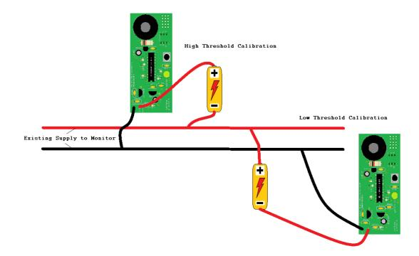
Looking at the diagram we can see how to use a single 1.5 volt battery to add and subtract 1.5 volts from an existing supply. Calibration of the high and low thresholds in this way gives a small margin around the voltage at the time of calibration.
