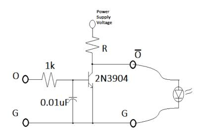
Also suppose that your supply  $(V_{PS})$  was 13.8V. We can calculate both the resistance value and the power value for R as follows:
