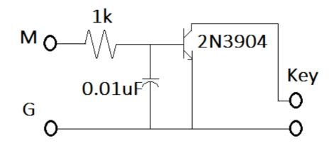
A code oscillator can be generally keyed by a simple straight key. A straight key is a simple switch that shorts two contracts. Here we are using the 2N3904 as an inverter and to provide enough key current to drive many code oscillators. Optical isolation might also be used but output current from the optical isolator may not be enough to directly drive the oscillator.
